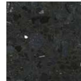
polished surface with black marble aggregates
