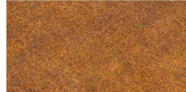
1. Appearance/shades of oxidized product at the time of delivery (approximately 2 months of oxidation).
