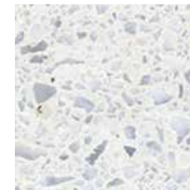
polished surface with white marble aggregate
