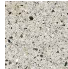
polished surface with granite aggregates
