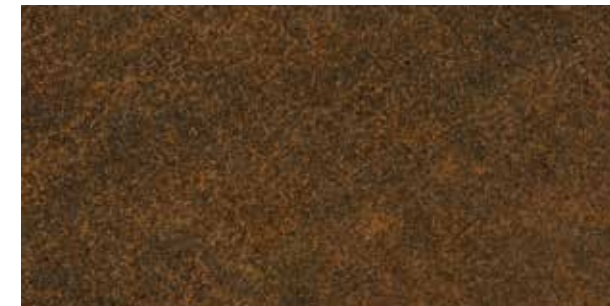
3. Appearance/shades of the product at the end of the period of oxidation after about 12/18 months of installation.
