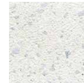
sandblasted surface with white aggregate
