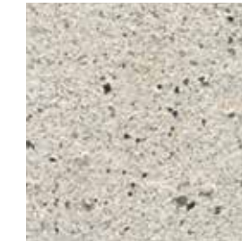
sandblasted surface with granite aggregates
